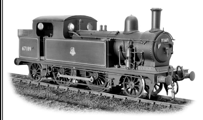
**Prototype.** This class was originally built by the GER from 1903. They were initially the mainstay of the London suburban service but later worked all over East Anglia, operating on many of the country branch lines. The class lasted until 1958.
